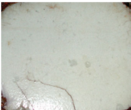
Figure 1 Air-cooled, PET-coated steel surface after exposure in the weathering chamber. [Color figure can be viewed in the online issue, which is available at www.interscience.wiley.com .]
